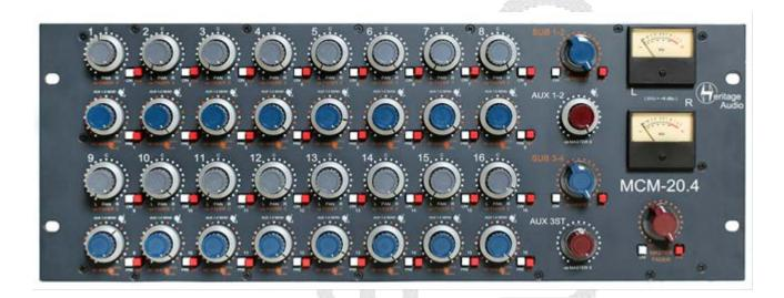
The front panel is laid out in 4 rows, 2 of 8 channels each featuring grey knobs and 2 with blue knobs carrying the aux sends sections. Further right are the related subgroup controls and aux sends master faders.
